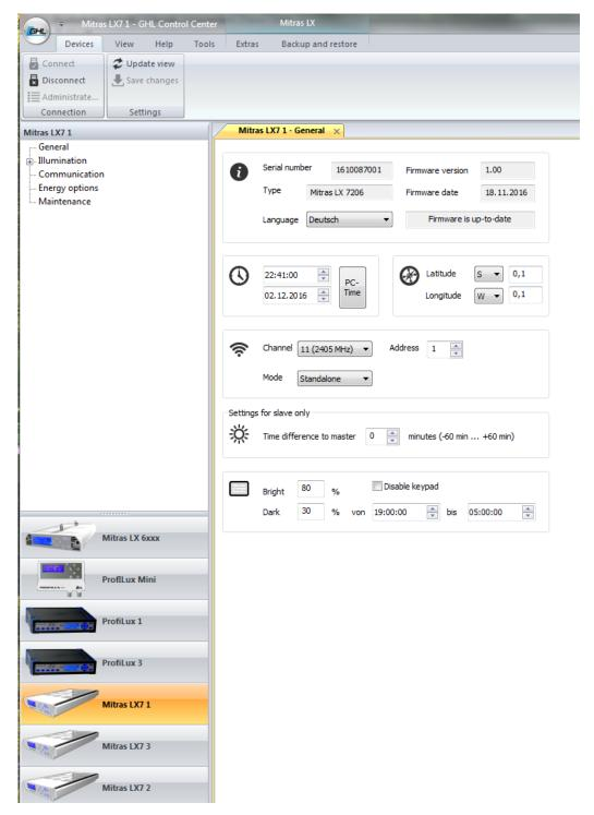
Once a connection has been successfully established, *GHL Control Center* examines the connected luminaire and displays the start screen. (Shown above)
