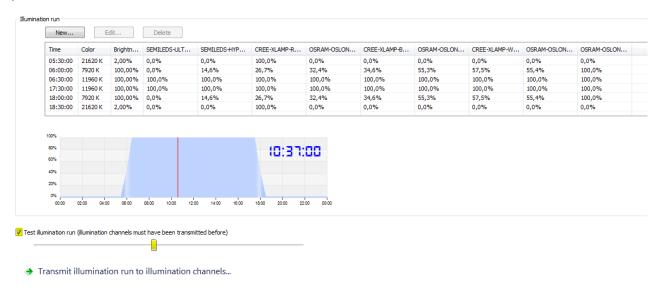
Activate the checkbox and move the slider. The illumination run can be followed directly on the luminaire.
