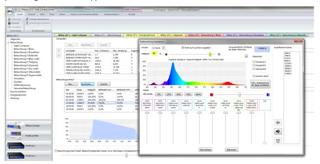
If you want to change the output color of the color channels, you can move them in the direction of blue or red using a slider. All color channels are automatically changed accordingly.
