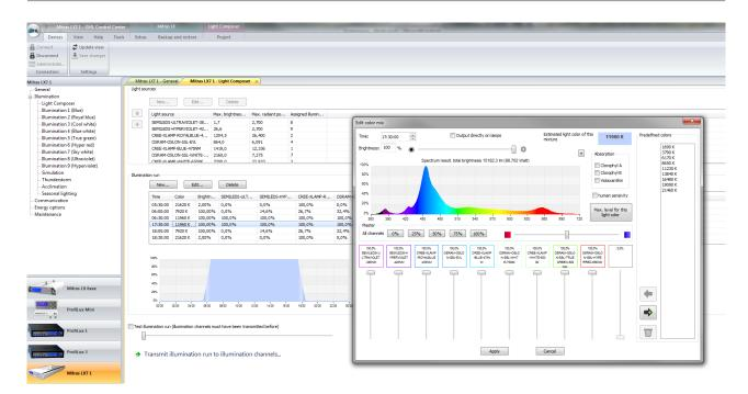
If you have ticked the checkbox "*Output directly on lamps*", you will see how the changed settings directly affect your connected luminaire(s). The display of the luminaire will now show "M" for manual lighting.
