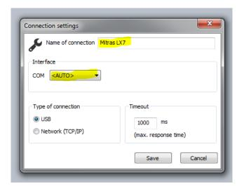
Enter any connection name (for example "Mitras LX7") and set the previously determined port (*COM4*) via the selection window (<Auto>). Press "*Save*".
