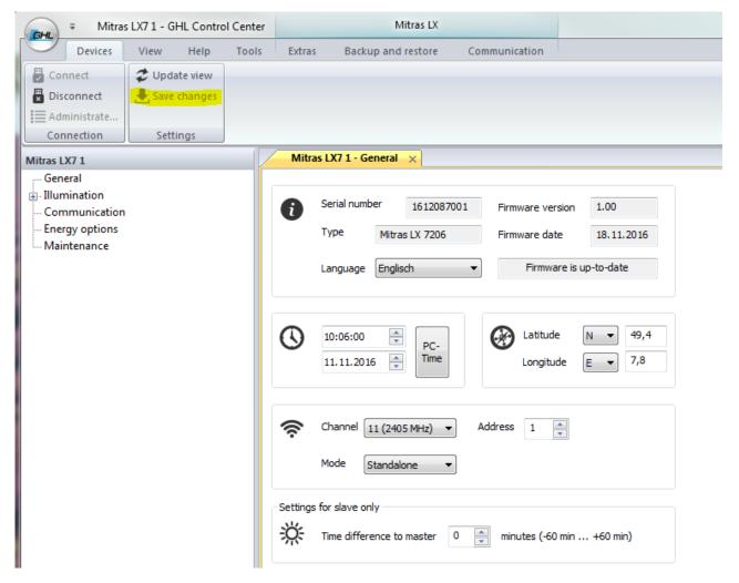
If your luminaire is connected to *GCC* and you make settings adjustments directly on your *Mitras LX7* at the same time, you have to transfer these to the GCC by pressing the "*Update view*" button.
